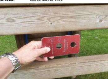
Finding: The item fails to meet the requirements of BS EN Action: Monitor - No remedial work recommended 1176 Part 1 4.2.7.2 for head and neck entrapment in the framework
